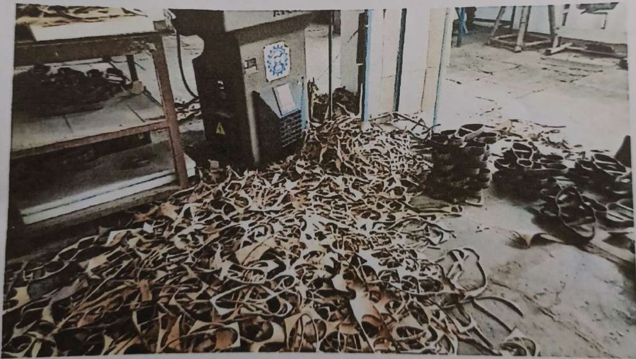
Figure 4 Material left over from cutting out soles for Kolhapuri chappal, at LIDCOM Kolhapur.
